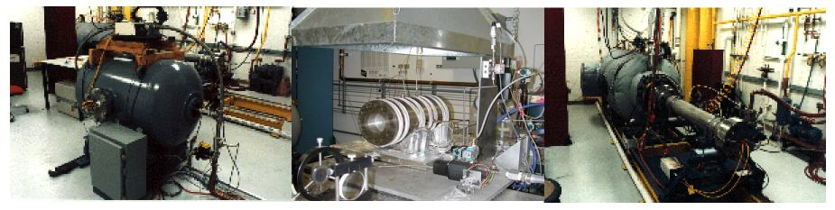
400 liter - flame propagation 600 cc -high pressure 1200 liter - transient jet & DDT
