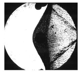
Projectile in T5 shock tunnel
